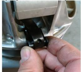
With stock clutches it is very common to see the side of the clutch wearing from the flyweight pivot end gouging into the aluminum, even with only low miles.
