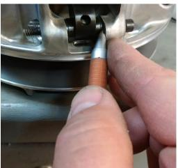
6)Install new primary spring into the clutch and re-install the cover onto the drive clutch (primary motor clutch). **Note: alignment marks.**
